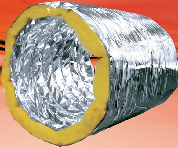
The **ASLI Insulated Flexible Air Duct (SHL-AFP)** is used widely in air-conditioning ductwork. The central core is permanently bonded to a coated spring steel wire helix that supports a thick blanket of fibreglass insulation, providing a double seal.
